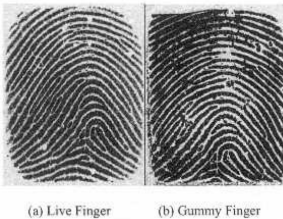
Figure 4.3 The sample images of fingers which derive from the same finger and were displayed on the screen when being scanned by the capacitive sensor of Device H.
