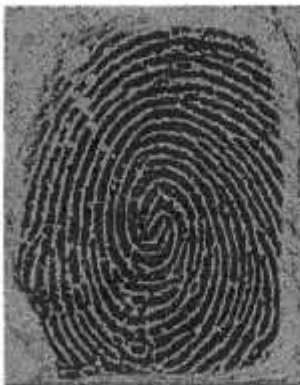
Figure 4.6 The Fingerprint image of the gummy finger, which was displayed by the system with Device H (equipped with a capacitive sensor).
